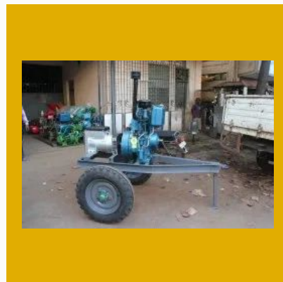
12 HP Diesel Engine Generator
